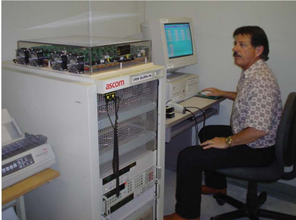
Front view of VRM Burn-In System
