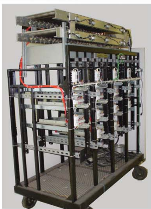
Rear view of duplicate Cart with resistive loads on top
