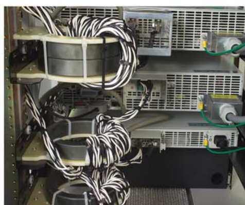
All Cabling through Ferrite Cores to minimize noise
