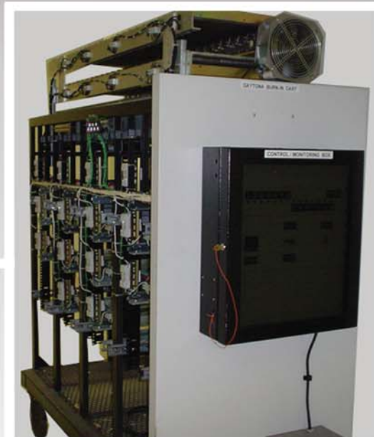
Side view of duplicate Cart with resistive loads on top
