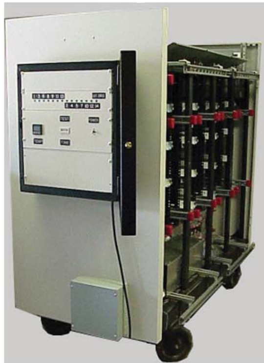
Side view of Life Test Burn-In Cart showing AC Input Power Control Box with Power Cycling Timer
