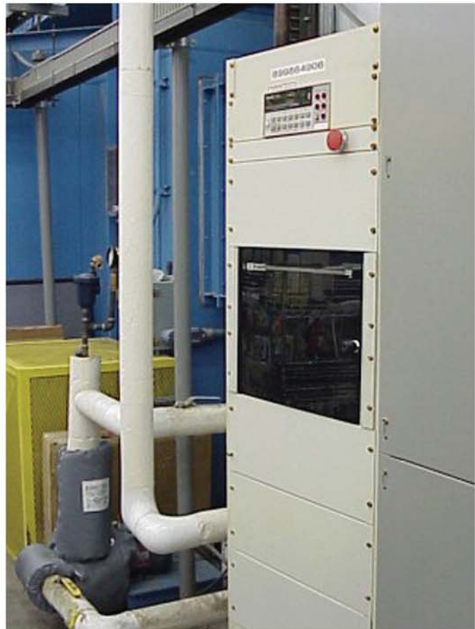
Front view of Burn-In Monitoring System Integrated with Thermal Chamber
