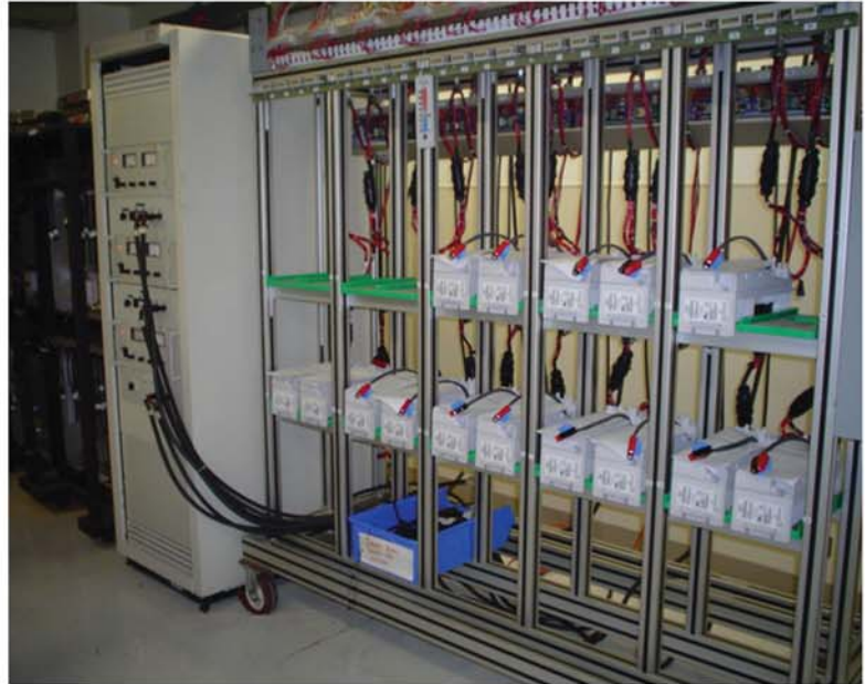
Front view of Burn-In Cart with 15 UUTs loaded and connected to the DC Input Power Cabinet
