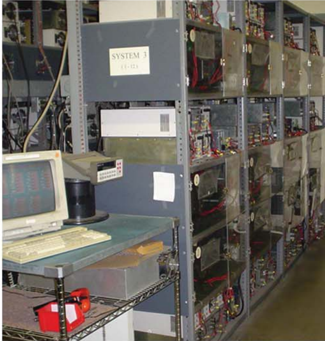
Side view of Burn-In System #3 and Burn-In Monitoring Software
