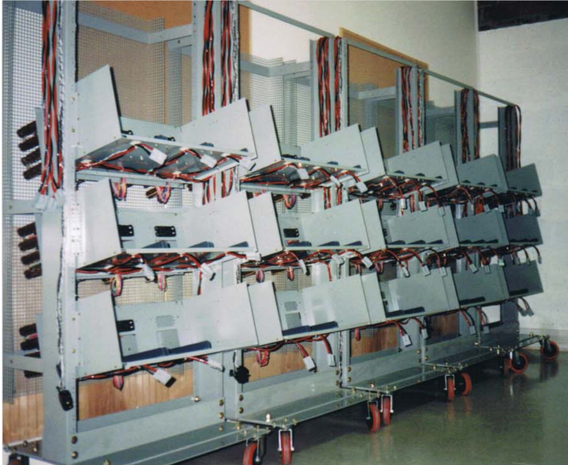
Front view of Multiple Burn-In Carts
