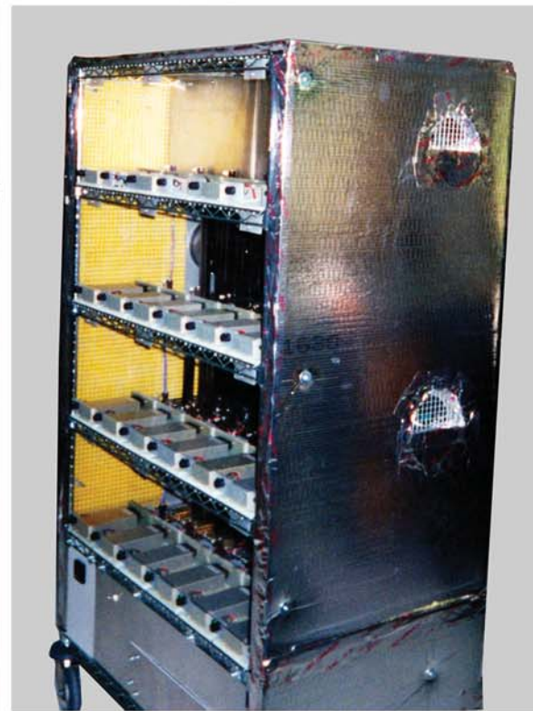
Heat Exhaust Fans on Side of Cart
