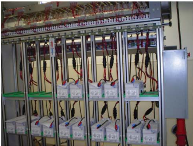
Close-Up of Burn-In Cart with AC Input Power Control Box on the side of the Cart
