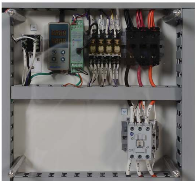
Close-Up of Thermocouple/Temperature Monitor to record temperature inside thermal chamber and disconnect Input Power to the UUTs if out of limits
